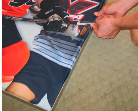
Lastly push in the middles of each side and work your way outwards
